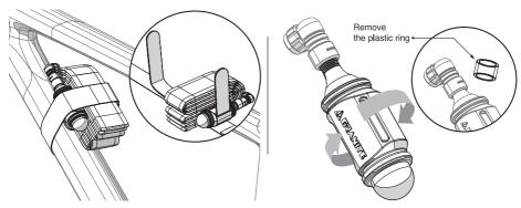
5. Open your tube's Presta valve. Push the inflator onto the valve. Carefully unscrew the canister and the air will start to flow.
